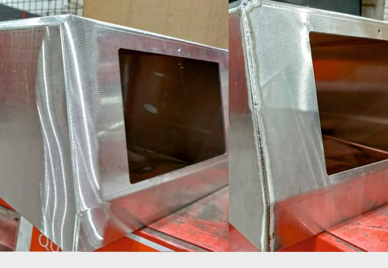
After the welding process, meticulous finishing techniques are used to ensure a flawless and aesthetically pleasing final product that meets the highest standards of craftsmanship. This includes precise dressing of welds and mirror polishing.
